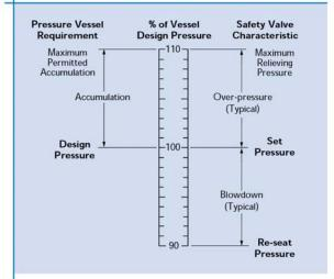
Note: System operating pressure must always be less than the re-seat pressure.
